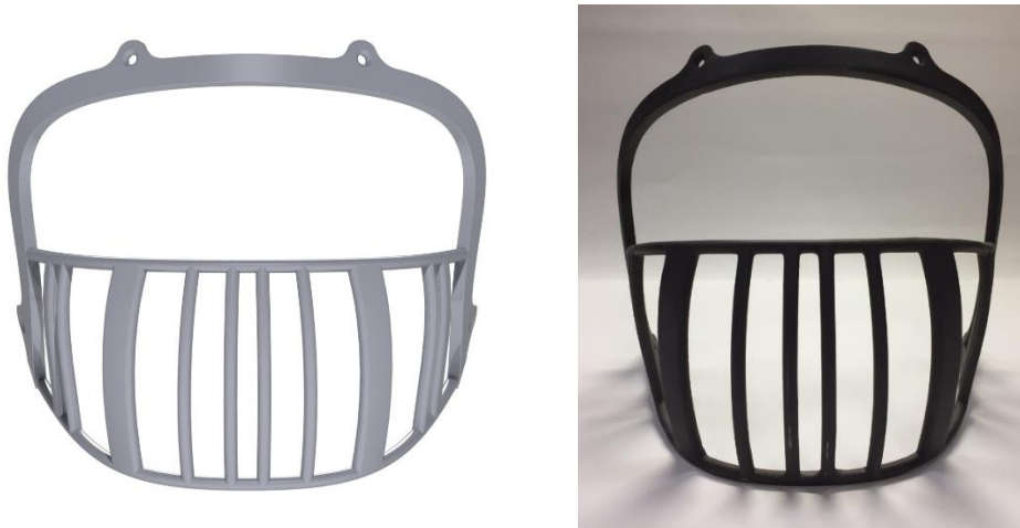
Figure 1.4 Johnson et al. [41] optimized faceguard SolidWorks model (left) and titanium cast (right).
